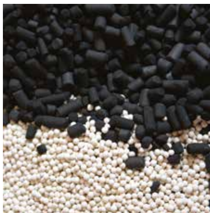
Active carbon and zeolite
